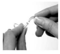
Hold the tube in one hand and the hearing aid hook in the other, twist and pull firmly apart.
