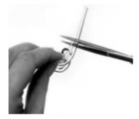
Use the old piece of tube as a measure for the new piece.
