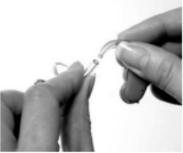
Push the end the hearing aid hook firmly inside the new piece of tubing.
