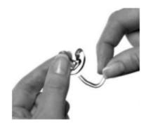
Pull the old piece of tubing out of the mould. **Keep this piece of tubing.**
