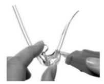
Using a sharp knife can create a closer cut. Place the mould down on a hard surface if using a knife.
