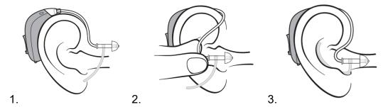
To insert a hearing aid with an **ear mould** see the images below. Hold the ear mould (1). Insert the mould into the top of the ear and the ear canal (2). Finally when the mould is secure and comfortable in the ear, place the hearing aid behind the ear (3).
