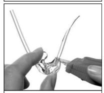
Using a sharp knife can create a closer cut. Place the mould down on a hard surface if using a knife.
