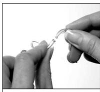
Push the end the hearing aid hook firmly inside the new piece of tubing.
