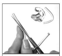
Cut the new piece of tubing to a long thin point.
