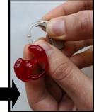
Push the earmould back onto the hearing aid.
