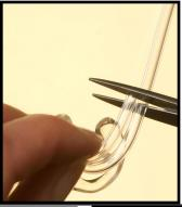
Place an old tube next to the new tube then cut the tubing.
