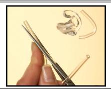
Cut a new tube at one end to make a point.
